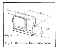
5. The recorder unit can be mounted on either a table-top, bulkhead or overhead. Make sure that the selected location is strong enough to support the unit under the conditions of continued vibration or shock which will be normally encountered on the boat. If necessary, appropriate reinforcement measures should be taken in the mounting area.
